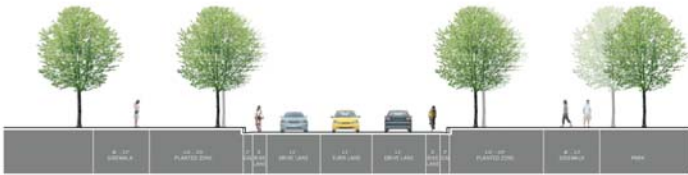
Figure 16.6B Section of typical three-lane Campus Greenbelt
