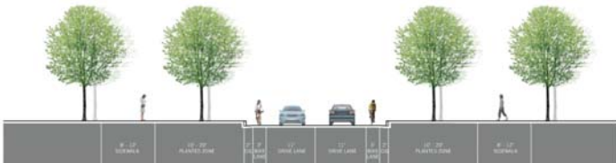
Figure 16.7B Section of typical two-lane Campus Greenbelt
