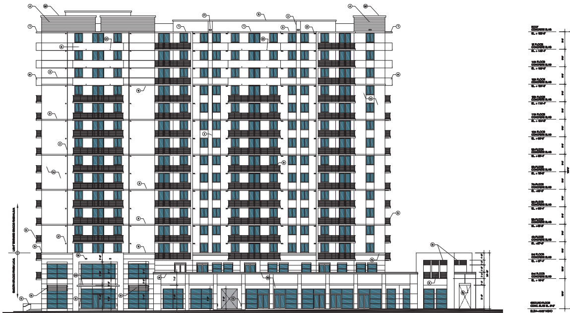
West Side Elevation Scale: 3/8" = 1'-0" NOTE: FOR TYPICAL NOTES AND SECTION MATERIAL LEGEND SEE SHEET A-A-2 FOR DIMENSIONS OF PARTS SEE ROOF PLAN (SHEET A-A-3) REFER TO STRUCTURAL DRAWINGS FOR DIMENSIONS OF FOOTINGS
